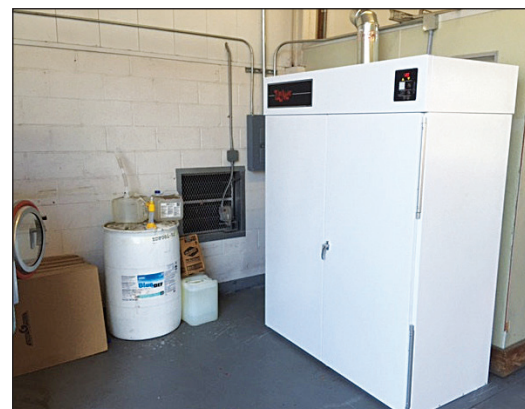
The department's new dryer cabinet allows it to dry fire hoses inside the station.
