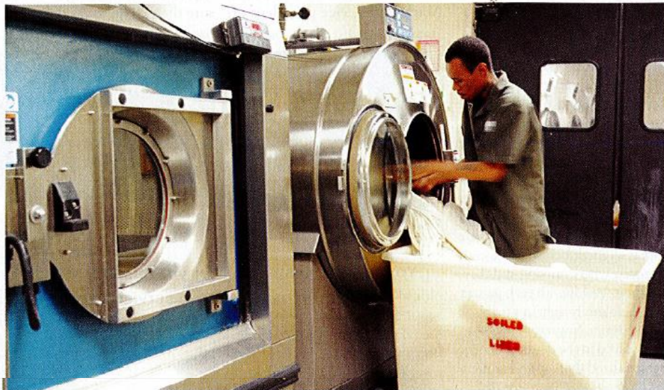
Lightly soiled linens don't need the same type of big-gun cycles as heavily soiled linens, experts remind. Many providers unknowingly waste chemicals, water — and money — by not adjusting washer's water levels.
